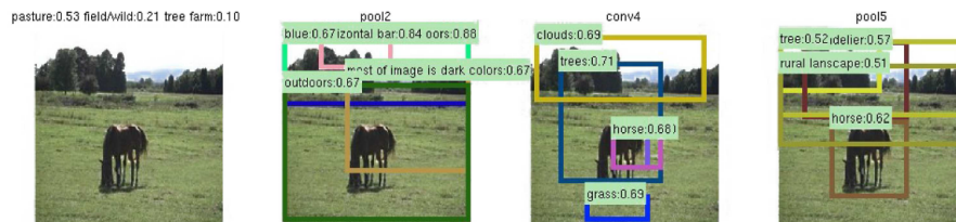
Figure 18: Interpretation of a picture by different layers of the Places-CNN (4.4.4 Places) using semantic tags given by humans. The first shows the final layer output of Places-CNN. The other three show detection results along with the confidence based on the units activation and the semantic tags.
