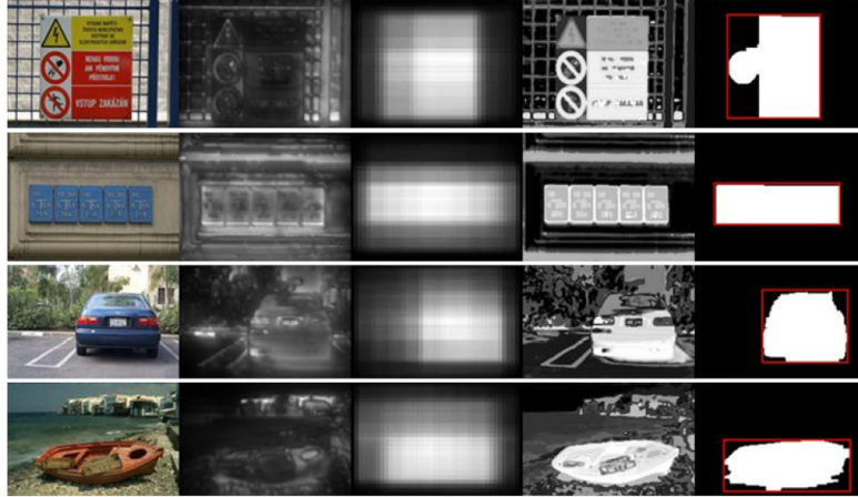
Figure 10: Examples of salient features. From left to right: input image, multi-scale contrast, center-surround histogram, color spatial distribution and binary salient mask by CRF.
